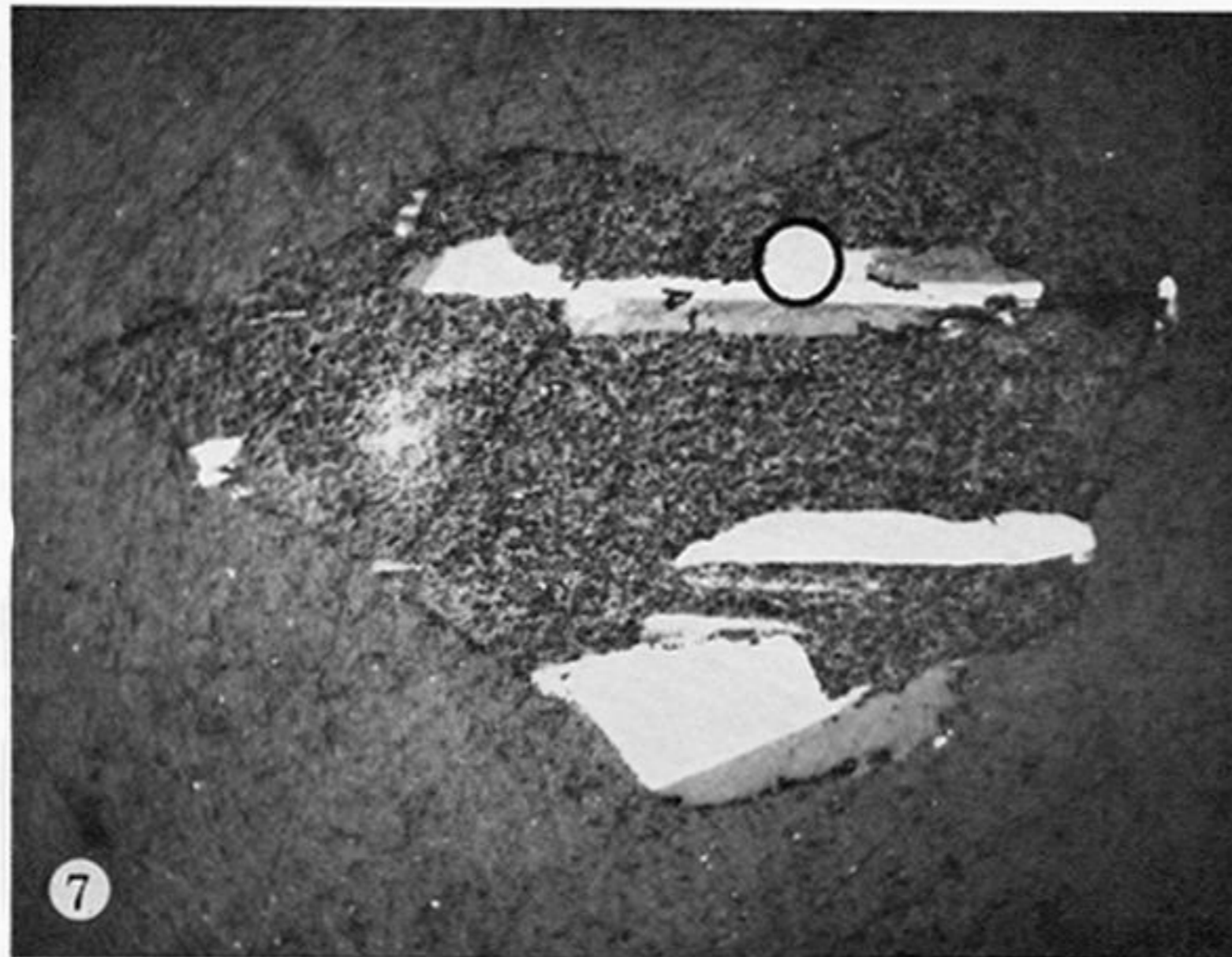
FIGURE 7. Serial section 4 of fragment L1, showing ilmenite, fayalite and silica. A small association of metal + troilite was encountered in the area indicated. Analyses in table 2. Reflected light, unetched. Field of view 190\ \mu\text{m} \times 240\ \mu\text{m} .
